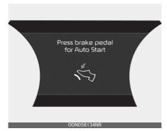
If you move the transmission lever from N to D (Manual mode) or R without depressing the brake pedal after stopping engine automatically, the engine does not restart automatically and a warning chime alarms. When this happens, press the brake pedal for auto start.
