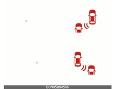
If a vehicle is detected within the boundary of the BCW, a warning light will illuminate on the outside rearview mirror and the Head-Up Display (if equipped).
