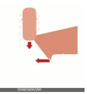
If the vehicle is parked rearward and the sensor detects the another vehicle in the rear area of the parking space, the system can warn or control braking.
