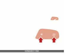
To change the rear fan speed, press the button () for higher speed, or press the button () for lower speed.
