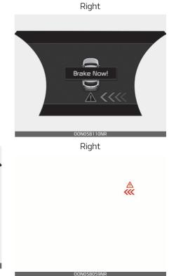
After brake control is activated, the driver must immediately depress the brake pedal and check the surroundings.
