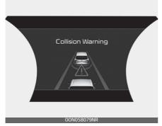
The warning message appears on the LCD display with a warning chime.
