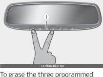
To erase the three programmed buttons (individual buttons cannot be erased):
