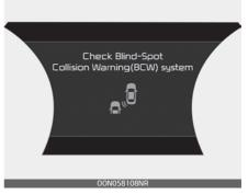
If there is a problem with the BCW, a warning message will appear and the light on the switch will turn off. The RCCW/RCCA will turn off automatically. RCCW and RCCA will not operate also if the BCW turns off due to malfunction. Have your vehicle inspected by an authorized Kia dealer.
