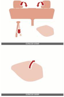
The headrest will fold down automatically when folding the seatback.
