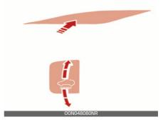
The sunroof will open only while pressing the control switch upward. Move the control switch forward to close the sunroof.
