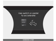
While the SCC is in operation, your vehicle stops behind the vehicle in front when it stops. The message is displayed on the cluster within 3 seconds after the stop and the system will be in the standby position.
