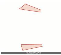
The BCW and BCA may not operate properly when driving where the heights of the lanes are different. In certain instances, the BCW/BCA may not detect the vehicle on a road with different lane heights (underpass joining section, grade separated intersections, etc.). Always pay attention to road and driving conditions, while driving.
