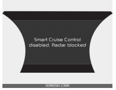
When the sensor lens cover is coverd with dirt, snow, or debris, the SCC operation may stop temporarily. If this occurs, a warning message will appear on the LCD display. Remove any dirt, snow, or debris and clean the radar sensor lens cover before operating the SCC.
