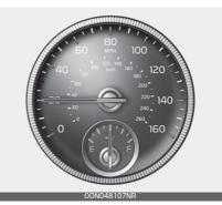
The speedometer indicates the speed of the vehicle and is calibrated in miles per hour (mph) and/ or kilometers per hour (km/h).
