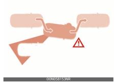
The BCA may activate the Electronic Stability Control (ESC) in accordance with a colliding possibility with an approaching vehicle while changing lanes.
