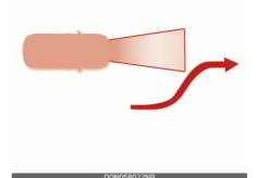
The FCA performance may be limited while driving upward or downward on a slope, and may not recognize the vehicle in front in the same lane. It may produce the warning message and the warning alarm prematurely, or it may not produce the warning message and the warning alarm at all.
