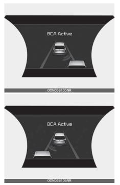
The BCA may apply braking power, when an approaching vehicle is detected within a certain distance next to/behind your vehicle.
