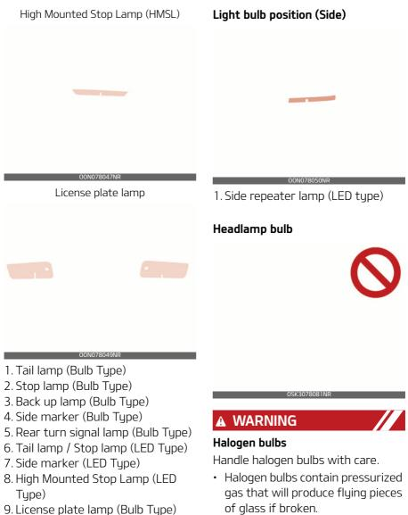
Always handle them carefully, and avoid scratches and abrasions. If the bulbs are lit, avoid contact with liquids. Never touch the glass with bare hands. Residual oil may cause the bulb to overheat and burst when lit. A bulb should be operated only when installed in a headlamp.
