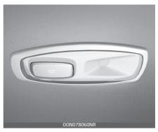
If the personal lamp (LED) does not operate, have the vehicle checked by an authorized Kia dealer. The LED lamps cannot be replaced as a single unit because it is an integrated unit. The LED lamps has to be replaced with the unit.
