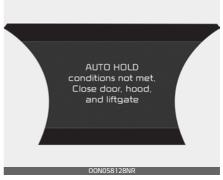
At this moment, press the [AUTO HOLD] button after closing the driver's door, engine hood and liftgate.
