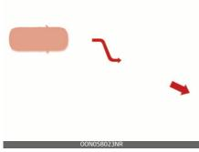
When driving in stop-and-go traffic, and a stopped vehicle in front of you merges out of the lane, the system may not immediately detect the new vehicle that is now in front of you.
