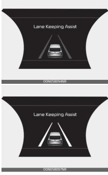
If the speed of the vehicle is over 40 mph (64 km/h) and the LKA detects lane markers, the color changes from gray to white.
