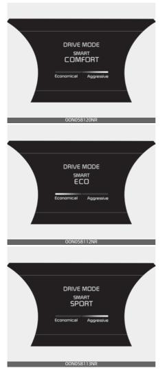
SMART mode selects the proper driving mode among ECO, COMFORT and SPORT by judging the driver's driving habits (i.e., mild or dynamic) from the brake pedal or the steering wheel operation.
