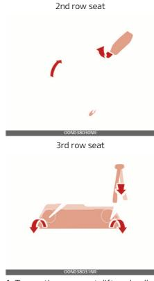
To use the rear seat, lift and pull the seatback backward. Pull the seatback firmly until it clicks into place. Make sure the seatback is locked in place. When you return the seatback to its upright position, always be sure it has locked into position by pushing on the top of the seatback.
