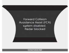
In this case, a warning message ("Forward Collision-Avoidance Assist (FCA) sustem disabled. Radar blocked") will appear to notify the driver.
