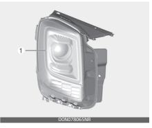
The LED lamps cannot be replaced as a single component because it is an integrated unit. The LED lamps have to be replaced with the unit. A skilled technician should check or repair the position lamp + DRL (LED), for it may damage related parts of the vehicle.
