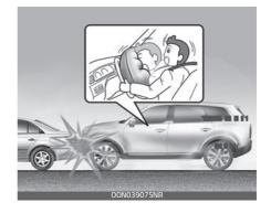
Front air bags are designed to inflate in a frontal collision depending on several factors, including the severity of impact of the front collision.
