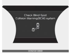
If there is a problem with the BCW, a warning message will appear and the light on the switch will turn off. The BCW will turn off automatically. The BCA will not operate also if the BCW turns off due to malfunction. In this case, have your vehicle inspected by an authorized Kia dealer.
