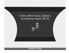
If there is a problem with the BCA, a warning message will appear. The BCA will turn off automatically. The BCW will still operate even if the BCA turns off due to malfunction. In this case, have your vehicle inspected by an authorized Kia dealer.
