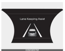
To see the LKA screen on the LCD display in the cluster, Tab to the ASSIST mode (
