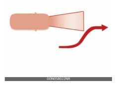
A vehicle which moves into your lane from an adjacent lane cannot be recognized by the sensor until it is in the sensor's detection range.
