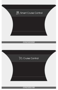
The driver may choose to only use the cruise control mode (speed control function) by doing as follows:
