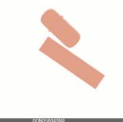
The BCW and BCA may not operate properly when driving on a curved road. In certain instances the system may not detect the vehicle in the next lane.
