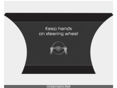
The hands-off warning appears when the system detects that the driver's hands are not on the steering wheel while the HDA is in work. (First warning: warning message, Second warning: warning message and warning sound)
