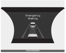
The warning message appears on the LCD display with the a warning chime. Additionally, some vehicle system intervention occurs by the engine management system to help decelerate the vehicle.
