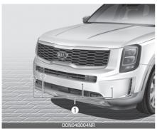
The sensing range and objects detectable by the sensors (1) are limited. Whenever moving while using the parking distance warning, pay as much attention to what is in front and behind you as you would in a vehicle without parking distance warning.
