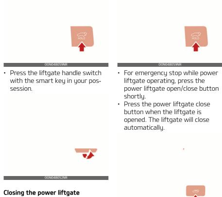
Press the power liftgate open/ close button for approximately one second when the liftgate is opened. The liftgate will close automatically.
