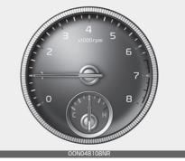
The tachometer indicates the approximate number of engine revolutions per minute (rpm).
