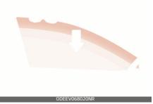
If the window detects the resistance while the power window switch is pulled up continuously, the window will stop upward movement then lower approximately 1 in (2.5 cm).
