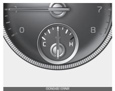
This gauge indicates the temperature of the engine coolant when the ENGINE START/STOP button or ENGINE START/STOP button is ON.
