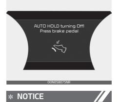
Engage the brake pedal when the above message appears for the Auto Hold and EPB may not activate. If the EPB is applied while Auto Hold is activated because of an Electronic Stability Control (ESC) signal, a warning will sound and a message will appear.
