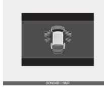
This warning is displayed if any door or the hood or the liftgate is left open. The warning will indicate which door is open in the display.
