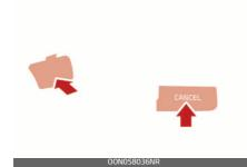
The SCC is temporarily canceled when the brake pedal is depressed or the CANCEL button is pressed.
