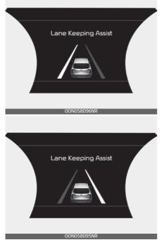
If the vehicle moves out its lane because steering torque for assistance is not enough, the line indicator of deviation direction will blink and the warning sound is provided.
