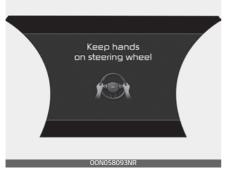
If you keep your hands off the wheel while driving with the LFA is in steering assist mode, the hands-off warning will be triggered.
