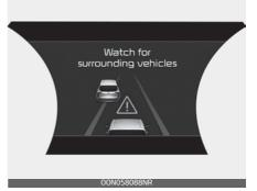
If the vehicle ahead (vehicle speed: less than 20 mph (30 km/h) moves to the next lane, the warning chime will sound and a message will appear. Adjust your vehicle speed for vehicles or objects that can suddenly appear in front of you by depressing the brake pedal according to the road and driving conditions.
