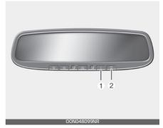
• Press the I button (1) to turn the automatic- dimming function on.
