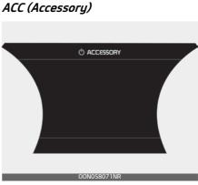
Press the ENGINE START/STOP button while it is in the OFF position without engaging the brake pedal.
