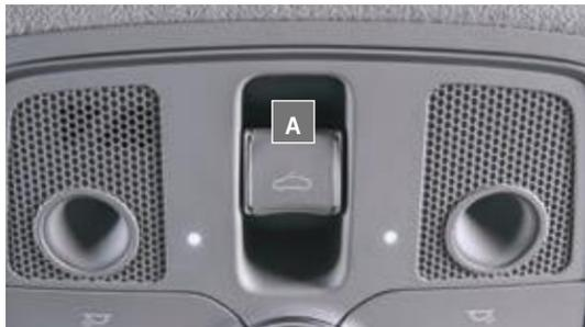
The Sunroof and Sunshade\* operation is controlled through a multidirectional switch/lever **A**, and the ignition needs to be in the ON position to operate the sunroof/sunshade.
