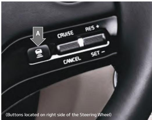
(Buttons located on right side of the Steering Wheel)
