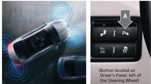
The Parking Assist System\*7 is a supplemental system that assists the driver by chiming if an object is detected within the sensing areas in the front or rear of the vehicle when parking or backing up.
