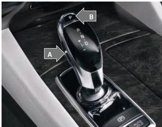
To shift into any gear from Park, depress the brake pedal, then press the Unlock button **A**, located on the side of the gear shift lever, and shift.
