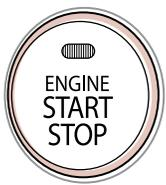
With standard key vehicles, you can turn the key to the accessory mode and utilize the electronic accessories without starting the vehicle. This is still possible with Smart Key-equipped vehicles. To do this, enter the vehicle with the Smart Key and push the ENGINE START/STOP button one time without depressing the brake pedal. This will put the vehicle in Accessory mode and the indicator will illuminate in yellow.
