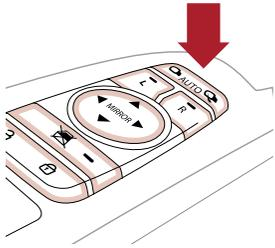
To fold or unfold the outside mirrors, press the folding mirror button as pictured.
