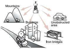
Satellite radio reception requires direct line of sight with the satellite transmitting the radio signal. Tunnels, bridges, covered parking, mountainous terrain, tall buildings, heavy foliage, and other obstacles may momentarily interrupt the signal. This is normal operation, and reception will be restored within a few seconds in an open, unobstructed area.
