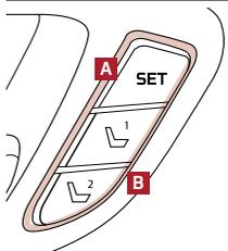
To store a seating position into memory, first place the gear shift into P (Park) while the ENGINE START/STOP button is ON. Then:
