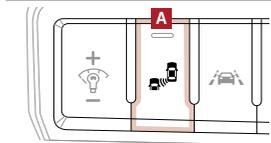
The BCW system uses radar sensors to detect vehicles in the blind spot, and alerts the driver before changing lanes. The light on the BCW button (A) will illuminate when turned ON. The outside rearview mirror warning lights will also illuminate for 3 seconds.
