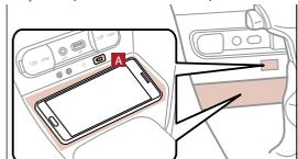
1. Place a compatible smartphone on the center of the charging pad.
