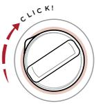
Tighten the cap until it clicks one time; otherwise, the Check Engine Light
