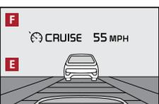
The Smart Cruise Control (SCC) system allows you to set the vehicle to maintain a speed so long as it is not limited by traffic. When traffic is encountered, the vehicle may be slowed to help maintain a set distance behind traffic detected ahead without the driver depressing the brake pedal.
