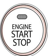
With standard vehicle keys, you can turn the key to the accessory mode and utilize the electronic accessories without starting the vehicle. This is still possible with Smart Key-equipped vehicles. To do this, enter the vehicle with the Smart Key and push the ENGINE START/STOP button one time without depressing the brake pedal. This will put the vehicle in Accessory mode and the indicator will illuminate in yellow.
