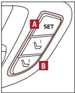
To store a seating position into memory, first place the gear shift into P (Park) while the ENGINE START/ STOP button is ON. Then:
