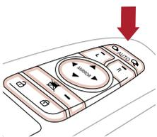
To fold or unfold the outside mirrors, press the folding mirror button as pictured.
