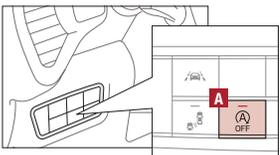
The ISG system is designed to help reduce fuel consumption by automatically shutting down the engine when the vehicle is at a standstill.
