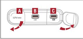
**Power Outlets A:** Use the power outlets for mobile phones and other devices designed to operate on a 12V (180W max.) power outlet.
