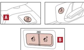
To get in and out of the 3rd-row seat, you can slide forward and fold down the 2nd row while pressing the One-Touch Slide and Fold buttons. Buttons are located on the seat cushion **A** and in the cargo area **B**. When stowing 3rd-row seats, it is best to use the One-Touch Slide and Fold button in the cargo area **B** to first stow the 2nd-row seats in order to prevent damage to 3rd-row seats.
