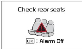
The Rear Occupant Alert can help alert the driver if the system detects a rear passenger has been left in the vehicle. The 1st alert will be a message on the Instrument Cluster. After the 1st alert, when the doors are locked and there is movement detected in the rear seats, the horn will sound for about 25 seconds.
