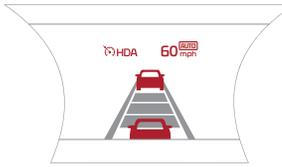
The Highway Driving Assist (HDA) system is designed to automatically adjust the speed of the vehicle to changing speed limits when driving on federal highways based on available highway speed information.
