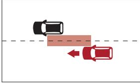
The Safe Exit Assist (SEA) system can help prevent passengers from opening their door after your vehicle has stopped when it detects a vehicle approaching from behind by displaying a warning message on the Instrument Cluster and sounding an audible warning.
