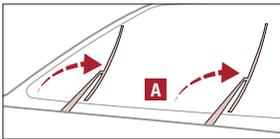
To inspect or replace the windshield wiper blades and to prevent damaging the hood, the blades need to be moved to the service position **A**.
