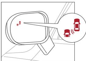
The BCA-R system uses radar sensors in the rear bumper to help monitor and warn the driver if it detects an approaching vehicle in the driver's blind spot area. It activates when the vehicle is traveling faster than 20 mph and will alert the driver if another vehicle is detected by the radar sensor.
