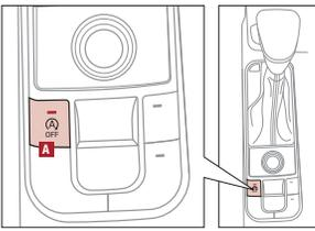
The ISG system is designed to help reduce fuel consumption by automatically shutting down the engine when the vehicle is at a standstill.
