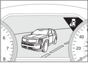
The Blind-spot View Monitor (BVM) system is designed to display the passenger-side rear blind spot areas in the Instrument Cluster LCD when the system is activated.
