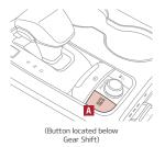
Auto Hold temporarily maintains the vehicle at a standstill even if the brake pedal is released. Auto Hold can be turned ON/OFF using the AUTO HOLD switch A located below the Gear Shift. Before Auto Hold will operate, the driver's door, engine hood, and trunk must be closed, and the driver's seat belt must be fastened.
