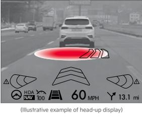
Augmented Reality Head-Up Display (HUD) is a semi-transparent display that projects a snippet of information from the instrument cluster and navigation system onto the windshield glass.
