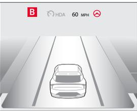
HDA is designed to adjust the speed of the vehicle when driving on limited/controlled access highways/freeways. The system can adjust the vehicle's speed based on available highway speed information. The automatic speed setting mode is designed to set the speed automatically by adjusting to the current speed limits of the highway the vehicle is traveling on.
