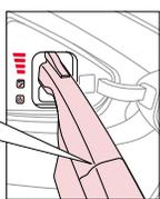
EV Charge Transfer / Vehicle to Load (V2L) allows you to use the vehicle's high-voltage battery to power electrical devices like home appliances or other electronic devices. V2L can also be used to charge items like electric bikes or another electric vehicle.
