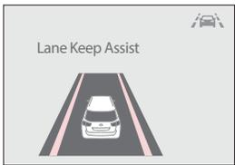
The LKA system guides the driver to keep the vehicle within its lane and provides steering inputs when the vehicle is about to deviate from the lane.
