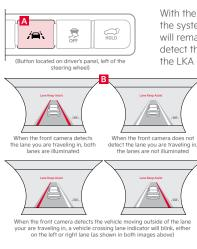
With the Engine Start/Stop button\* in the ON position, press the Lane Safety button A to turn the system ON or OFF. Once ON, the instrument cluster indicator will initially illuminate white. It will remain white when the vehicle is traveling slower than 40 mph or when the system does not detect the lane markers. When the system detects the lane markers and can assist the steering, the LKA icon will illuminate green.
