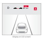
NSCC can automatically adjust the SCC's set vehicle speed according to speed limits and known curves on limited-/controlled-access highways using information from the Navigation System.
