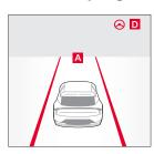
LKA is designed to detect the lane markers on the road and help alert the driver or assist in steering to potentially help keep the vehicle in the lane. LFA is designed to help the vehicle stay centered in its lane A by monitoring the detected lane markings ahead and adjusting the steering.
