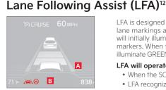
LFA is designed to help the vehicle stay centered in its lane A by monitoring the detected lane markings ahead and adjusting the steering. Once ON, the Instrument Cluster indicator will initially illuminate WHITE. It will remain WHITE when the system does not detect the lane markers. When the system detects the lane markers and can assist the steering, the LFA icon will illuminate GRFFN B
