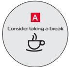
Driver Attention Warning (DAW) is designed to alert the driver if it detects inattentive driving patterns and, in certain situations, can give a warning signal to take a break. A message, "Consider taking a break" **A**, will appear on the display, and a warning will sound to suggest the driver take a break.
