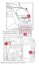
From outside of the vehicle: Open by pressing the Liftgate Release button A on exterior of the Liftgate, and close by pressing the Power Liftgate Close button B.
