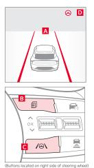
LKA is designed to detect lane markings (or road edges) and can warn the driver if the vehicle leaves the lane without using the turn signal and can, in certain circumstances, assist with steering to prevent the vehicle departing from its travel lane. LFA is designed to help ensure that the vehicle stays centered in its lane A by monitoring the detected lane markings ahead and vehicles on the road, and may provide steering inputs.
