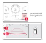
SVM is a parking assist system that shows the areas around the front, rear, left, and right sides of the vehicle, as well as a 3D view of the vehicle via the four cameras that's displayed onto the infotainment screen.
