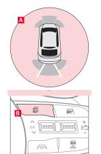
PCA-R is designed to detect certain objects/pedestrians behind the vehicle and issues an audible warning and/or applies emergency braking to help reduce the possibility of a collision when the vehicle is in reverse. When PCA-R activates, lines appear behind the vehicle image A in the Instrument Cluster.
